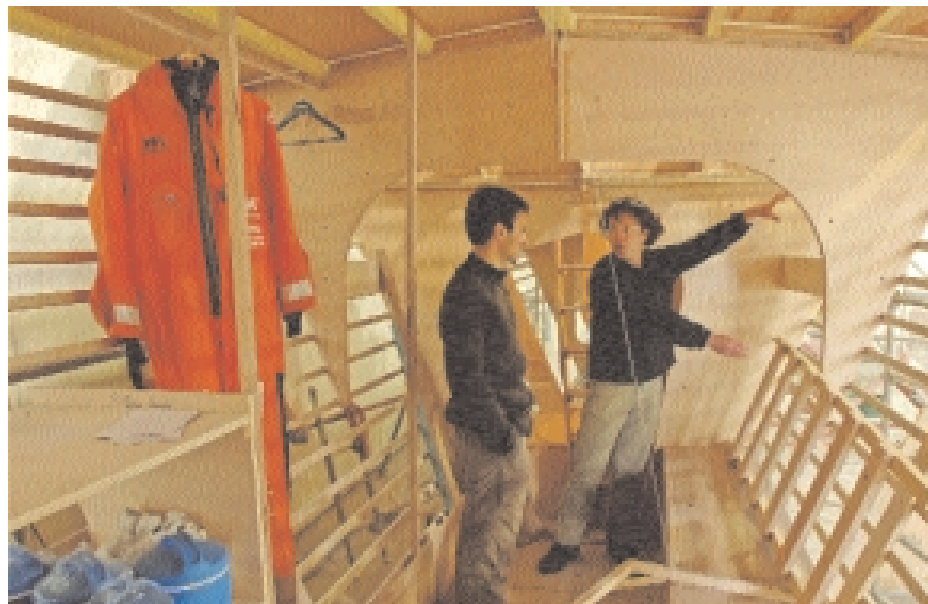
Inside the scale 1 fake central hull, made to pre-arrange deck and interior layout.
